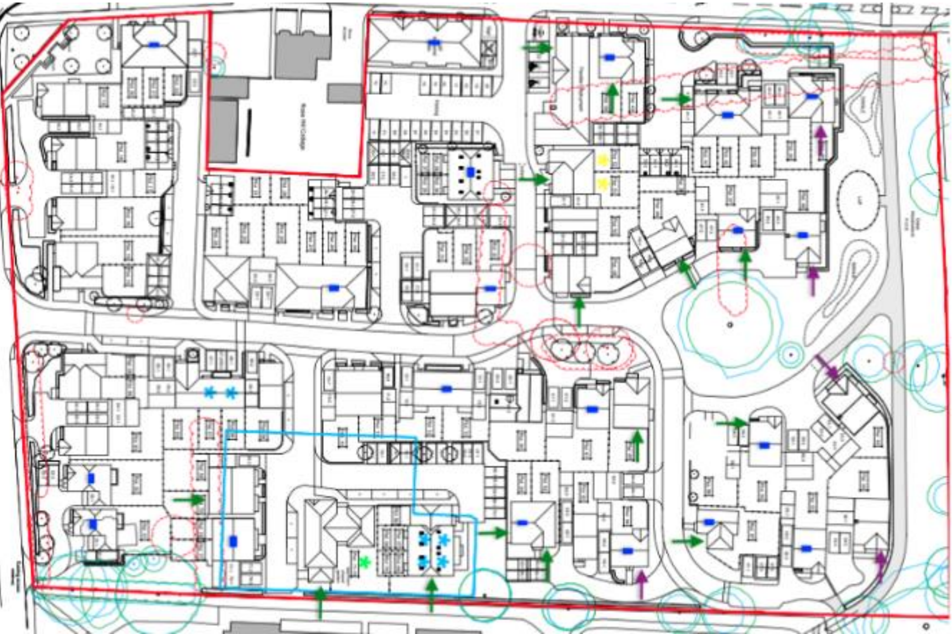
Biodiversity enhancements Bats- Habitat box = Green, Bat box = Purple, Bat tiles =Blue
